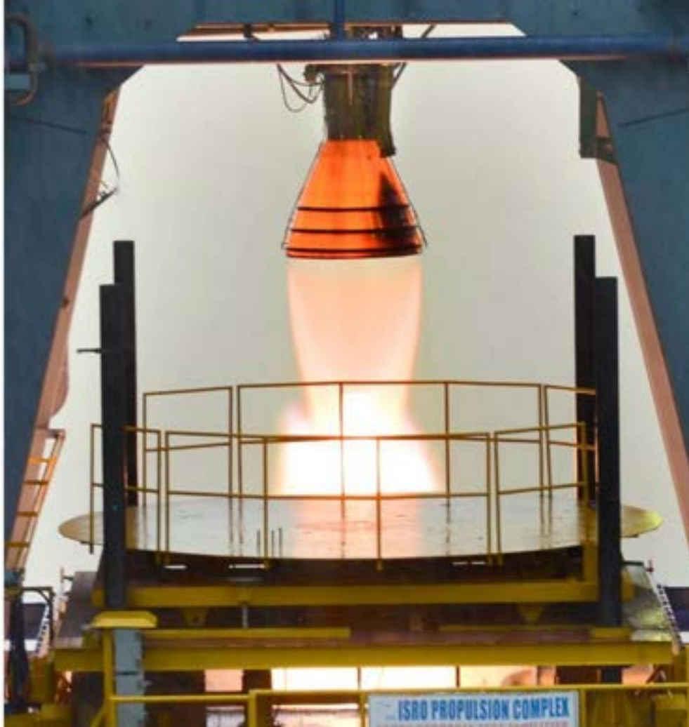
Fig.2. Photo of the testing of the Vikas Engine - the workhorse liquid rocket engine used to power the second stage of the ISRO's trusted PSLV.
